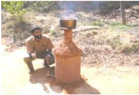
Volatiles being used to heat water in Charcoal-based kiln
