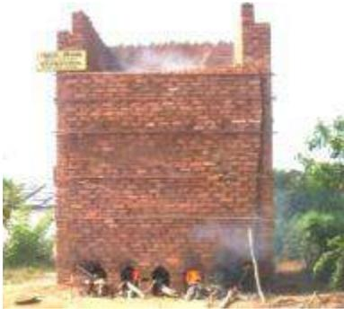
The improved brick kiln has been developed to make good quality conventional bricks with reduced quantity of fuel. Bricks are made in the informal sector in conventional clamp kilns. The capacity of these conventional clamps is about 40,000 bricks per batch. This means that the working capital required by a small brick maker is high. To address the problem Prof Jagadish of Gramavidya developed a fuel efficient brick kiln with a capacity of 12,000 bricks per batch.
