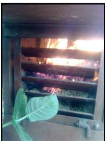
*Combustion chamber for loose biomass*
