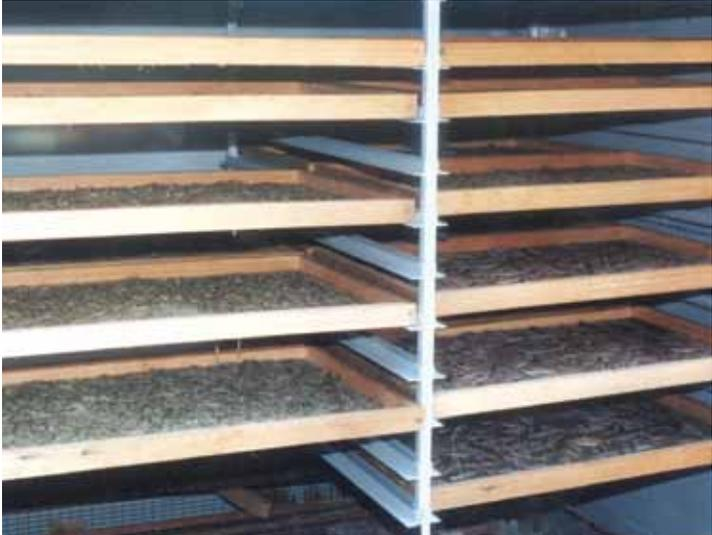
Fuel efficient biomass dryer in operation.
