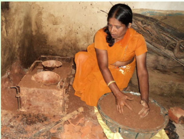
Katayani, TIDE's stove builder, constructing a smokeless
