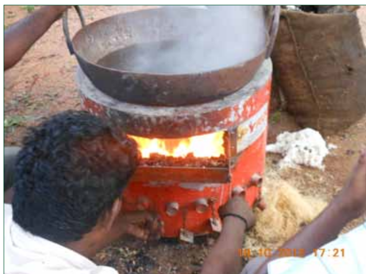
Figure 9: Loose biomass stove in use
