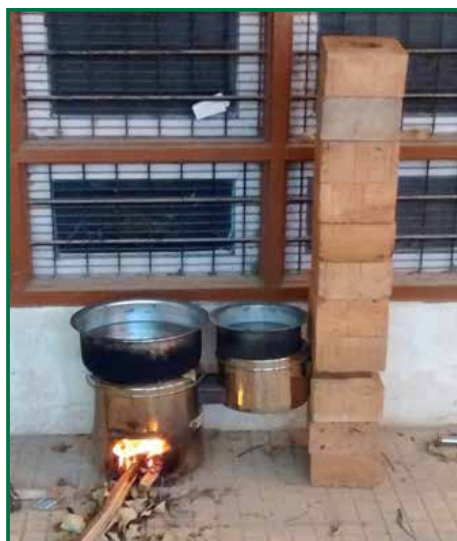
Developed adobe brick based chimney as alternate to ce- ment pipes
