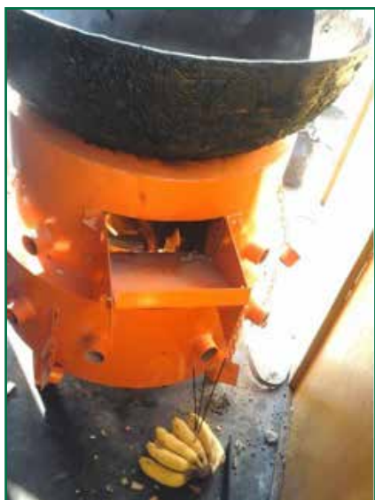
Sloping grate fuel feeding port in PYRO stove 54 cm
