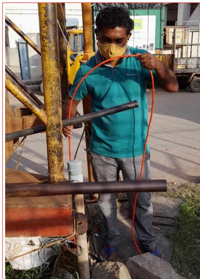
VIDEO LOGGING – BORE WELL No. 2
